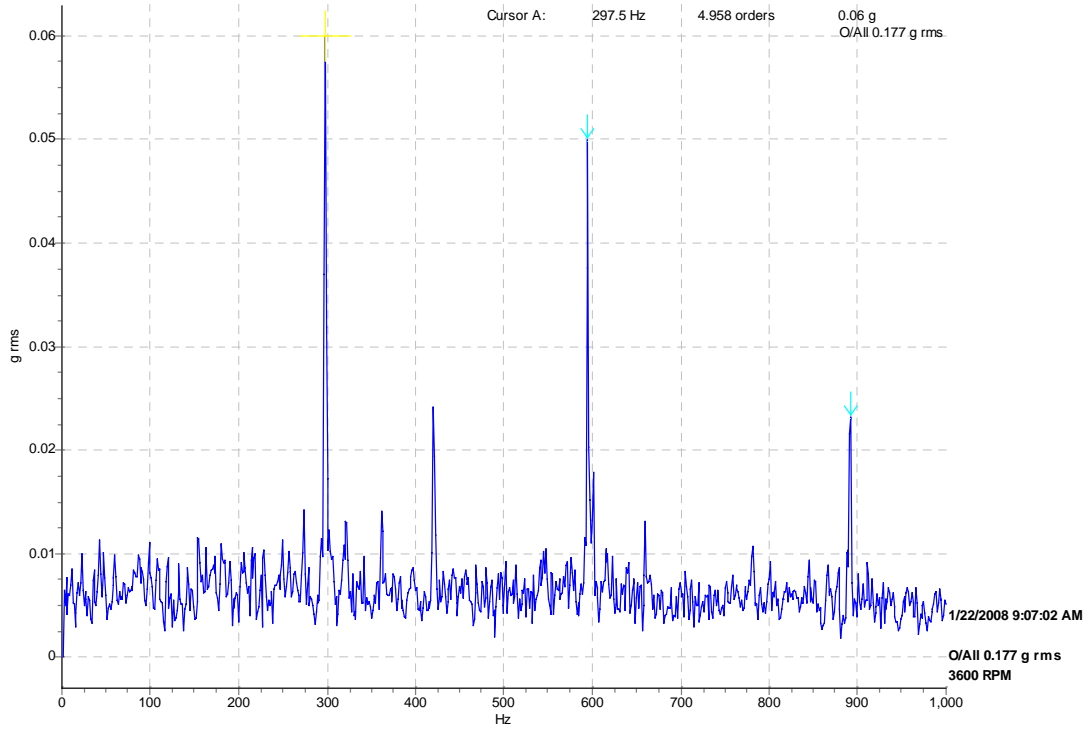
CH-2 - Motor Outboard - Axial - Demod (2-10kHz) 1000 Hz 1/22/2008 10:25:23 AM
