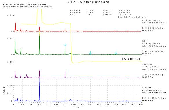
Very good 1xrpm levels seen in the motor outboard readings. Less than .05 ips noted.
