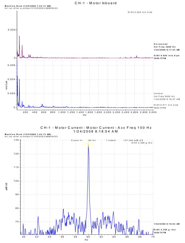
No faults noted in the motor current readings!
