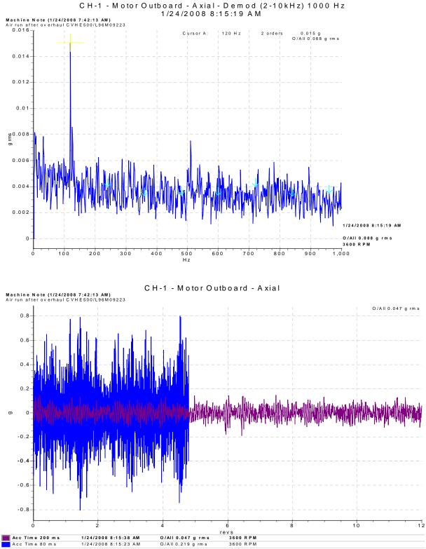
Axial waveform levels are below the nominal 2 G pk for the higher frequency and less than the nominal 1 G pk for the lower frequency range.
